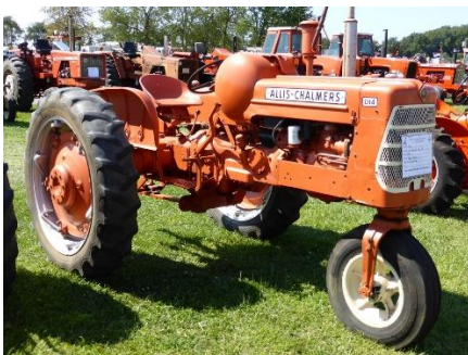
This is a rare D-14 propane 'High Clearance' with rear axle extensions and 16" front tire.
