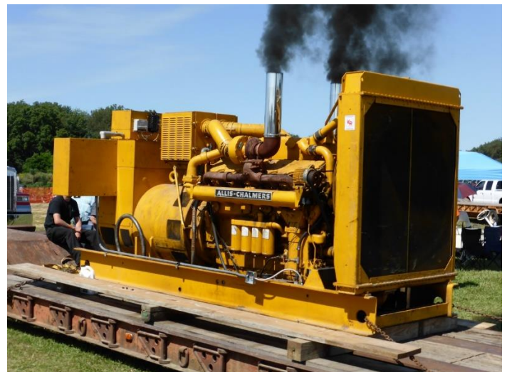
This is a V-12 '900 hp.' standby generator that was donated by Allis-Chalmers to the new Harvey Illinois hospital. 58 of these engines were hand built in the tool room of the A-C Harvey engine plant in the early 1970's. This engine was discovered two weeks before it was scheduled to be removed and scrapped.
