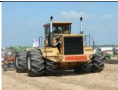
Feature tractor was a Rite-Way 750 powered by a Detroit 12V71 TT that had been tuned up to 850 hp. It plowed with a 15 furrow plow.
