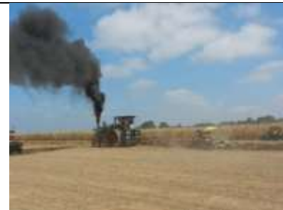
110 HP Case steam engine pulling a modern 10 furrow plow in hard dry ground.
