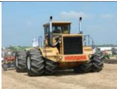
Feature tractor was a Rite-Way 750 powered by a Detroit 12V71 TT that had been tuned up to 850 hp. It plowed with a 15 furrow plow.
