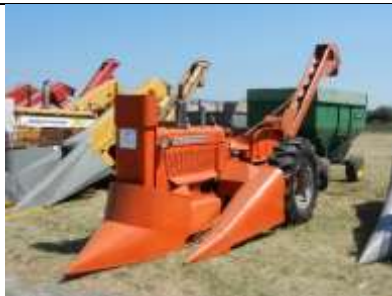
D-17 with mounted picker ready for the field.
